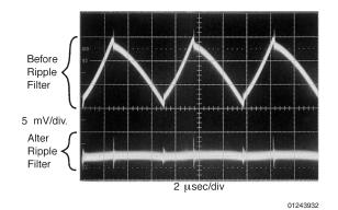
FIGURE 17. Post Ripple Filter Waveform
