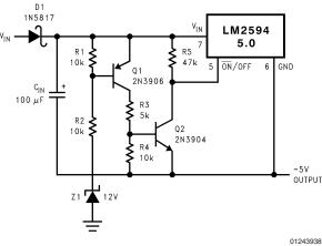
This circuit has an ON/OFF threshold of approximately 13V.
