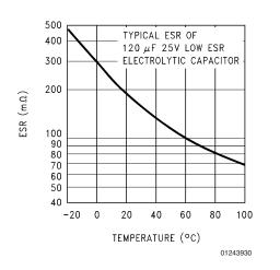
FIGURE 15. Capacitor ESR Change vs Temperature
