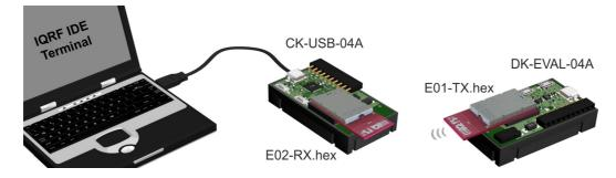
See Basic examples E01-TX, E02-RX, ... in IQRF Startup Package.
