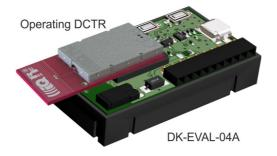
USB connector is intended just for accumulator charging but not for USB connectivity.
