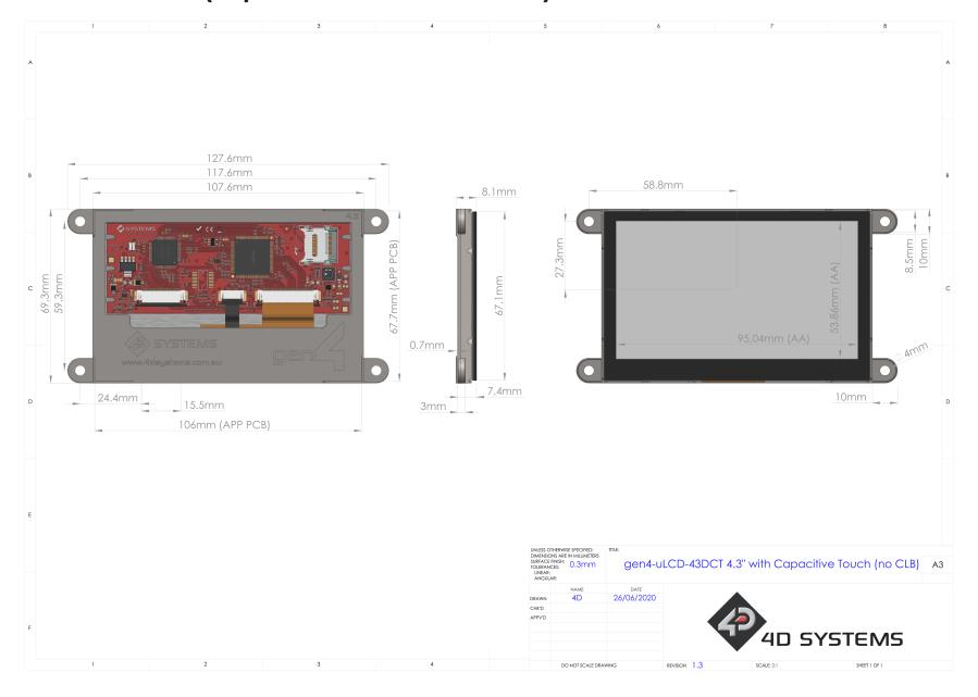
gen4-uLCD-43D Series Schematic Details (HW REV 1.2)
