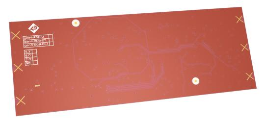
Where the Application PCB is shown to sit in under the Application PCB Support section; can house a small metal shield of the same size. This shield is used instead of, or underneath an Application PCB, to aid the onboard electronics in the prevention of potential RF or EMI signals.
