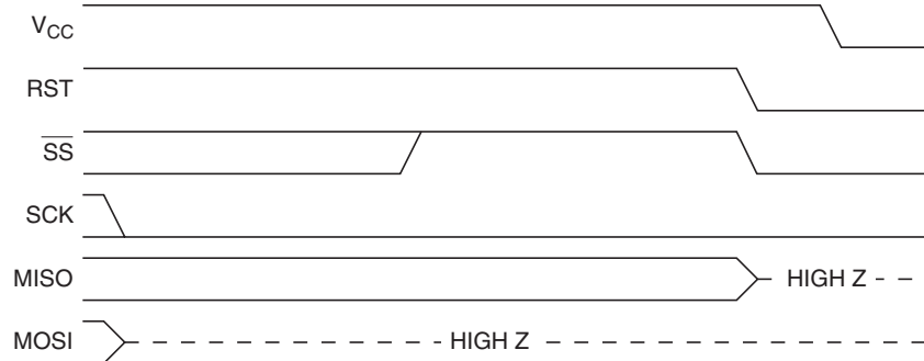
Figure 23-23. Serial Programming Power-down Sequence
