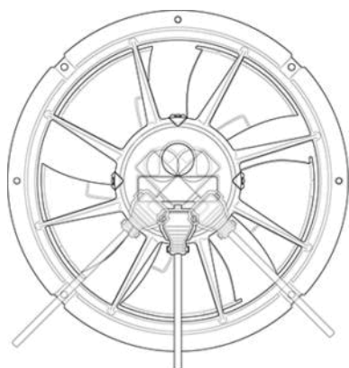
Fig. 2: Cable routing for fans installed upright. The cables must always be routed downward.
