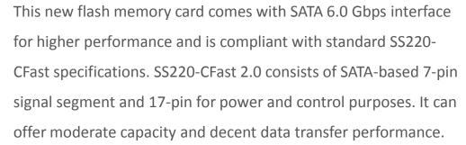
For power efficiency, this new flash memory card leverages the technological benefits of SATA Revision 3.1 specifications, including Device Sleep. That will greatly reduce power consumption when the device is not in operating mode. For data integrity, the SS220-CFast card is built with ECC engine correcting up to 40-bit.
