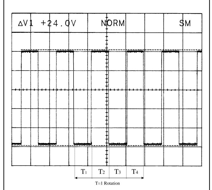
T=T1+T2+T3+T4 =(1 Rotation) T1=T2=T3=T4= $\frac{60}{4 \times \text{rpm}}$
