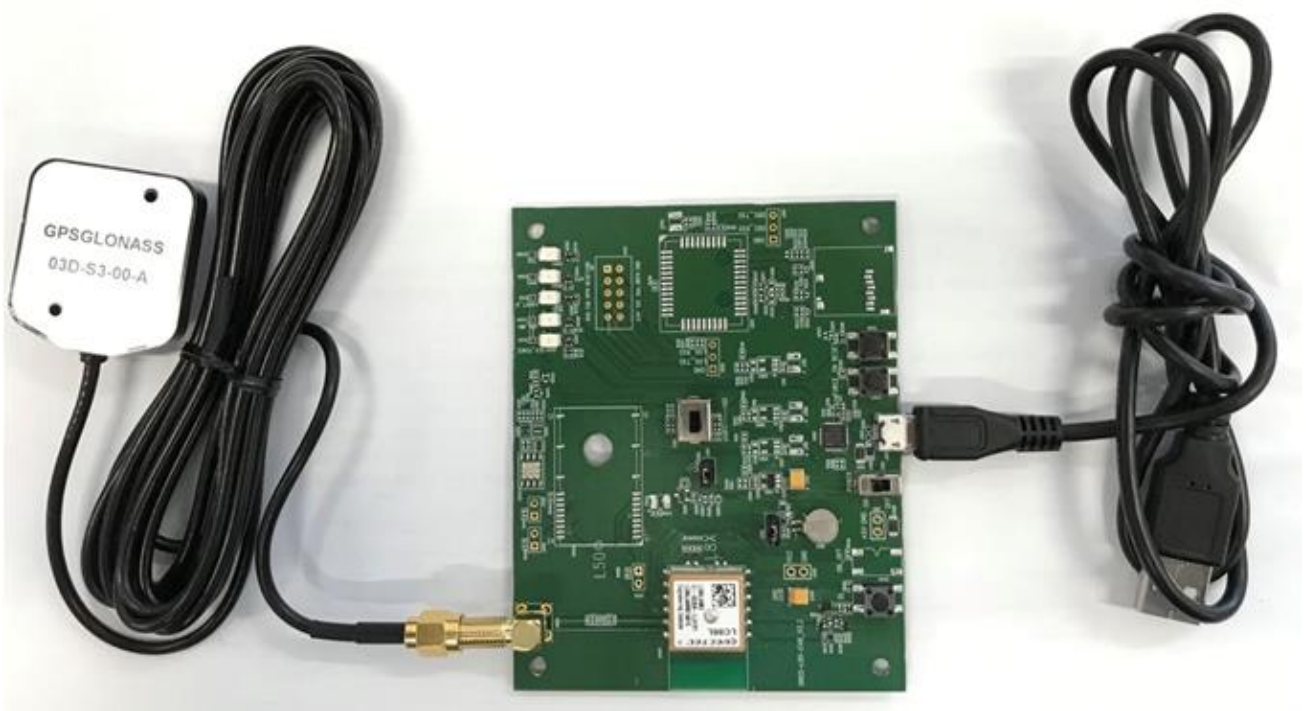
Figure 3: LC86L EVB and Accessories Assembly
