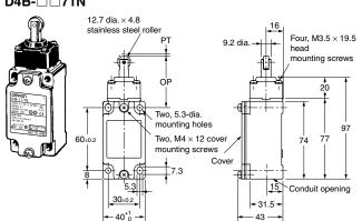
Note:Omitted dimensions are the same as those for the Roller Lever Type Models. D4B-1 N and D4B-5 N have a PG13.5 conduit opening. D4B-200N and D4B-600N have a G1/2 conduit opening. D4B-300N and D4B-700N have a 1/2-14NPT conduit opening.
