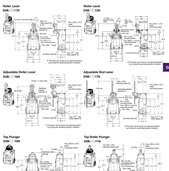
Note: Unless otherwise specified, a tolerance of ±0.4 mm applies to all dimensions. \*The lever can be set to any desired position by turning the operating position indicator.
