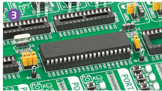
Figure 4-5: Properly placed microcontroller will have equally leveled pins.
