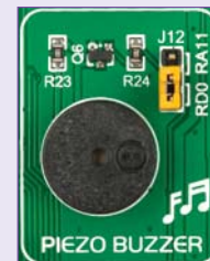
Figure 19-2: Use jumper J12 to connect Piezo buzzer on R20 or RA11 pin
