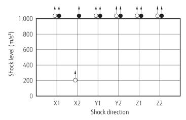
Shock application time: 6±1ms, half-sine wave Test material: coil energized and de-energized Shock direction: see diagram below Detection level: chatter > 1ms
