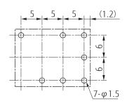
Tolerance of PC board mounting hole layout: ±0.1 unless otherwise specified.
