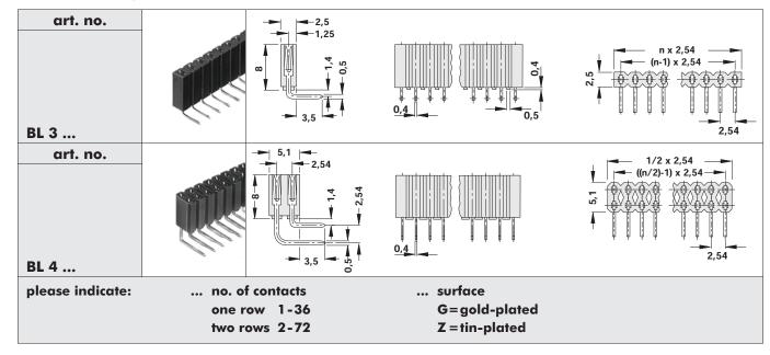
V-notches permit breaking! Therefore any required number of contacts is available.
