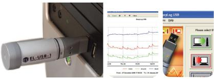
On inserting a battery the Red then Green LED will flash in turn for approximately 2 min, while the logger stabilises. Do not connect to the USB port of a computer untill this has finished.
