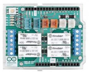
The **Arduino 4 Relays Shield** is a solution for driving high power loads that cannot be controlled by Arduino's digital IOs, due to the current and voltage limits of the controller. The Shield features four relays, each relay provides 2 pole changeover contacts (NO and NC); in order to increase the current limit of each output the 2 changeover contacts have been put in parallel. Four LEDs indicate the on/off state of each relay.
