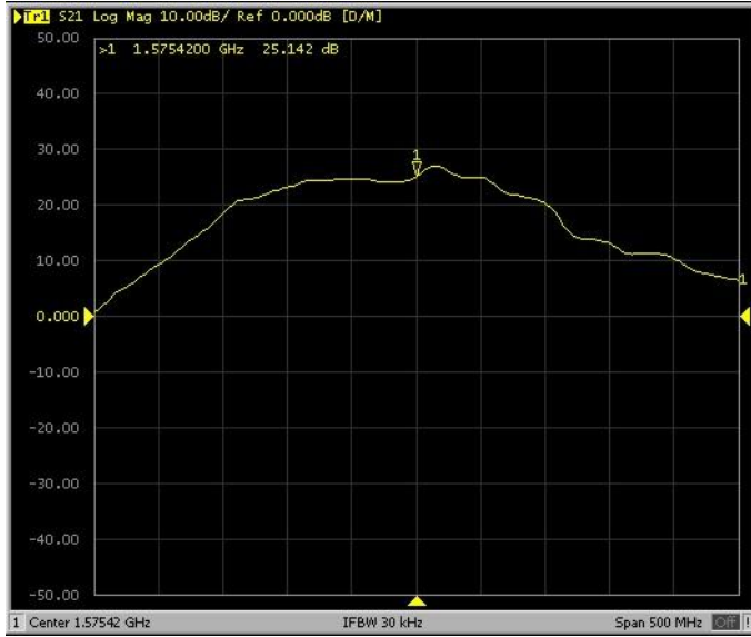
Tested with 3m cable length - RG174 with C20N
