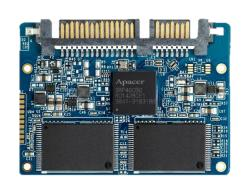
For data efficiency, the internal controlling unit of the SSD is engineered with DRAM for enhanced random performance. In regard of reliability, the drive comes with various implementations including powerful hardware ECC engine, power saving modes, wear leveling, flash block management, S.M.A.R.T., TRIM, and power failure management.
