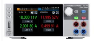
When the power supply is in constant voltage mode, the numbers and the keys are green. Red is used for constant current mode. The output key lights up blue to indicate that the channels are switched on (active).
