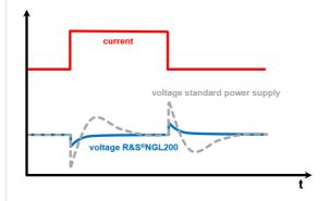
During challenging load conditions, most power supplies react with slow recovery times and overshoots. Specially developed circuits in the R&S\*NGL200 series achieve a load recovery time of  $< 30~\mu s$  with minimal overshoot, making them perfect for supplying sensitive components
