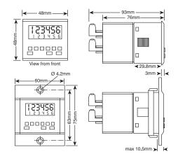
The count inputs are opto-isolated and can be sink (NPN) or source (PNP). The count is on the main display and the preset value is on the subsidiary display. Reset can be remote, manual or automatic with a manual over-ride option.
