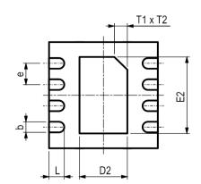
Figure 7 Dimensional drawing of STS3xA-DIS sensor package
