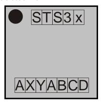
**Figure 6** Top View of the STS3xA-DIS illustrating the laser marking.
