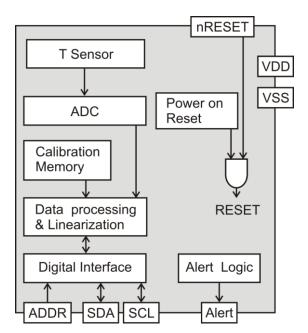
**Figure 1** Functional block diagram of the STS3xA-DIS. The CMOSens<sup>™</sup> technology allows providing for a fully calibrated I<sup>2</sup>C signal.
