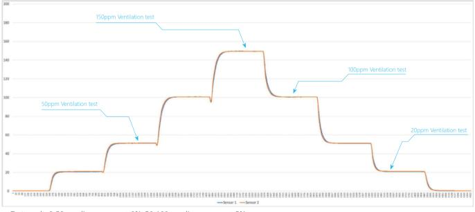
Test result: 0-50ppm linear error <± 3%; 50-100ppm linear error <± 5%;
