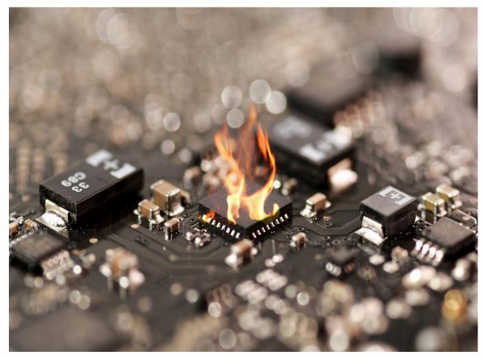
What is meant by a thermal runaway or the thermal damage of power semiconductors: A thermal runaway refers to the overheating of a technical apparatus due to a self-reinforcing process that generates heat. This damage usually causes the destruction of the apparatus and often leads to a fire or explosion.
