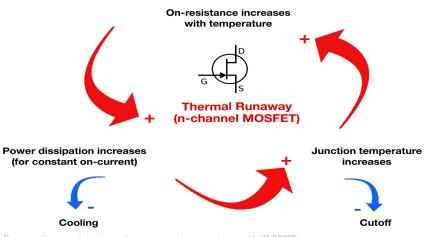
Cause diagram for thermal runaway at an n-channel MOSFET
