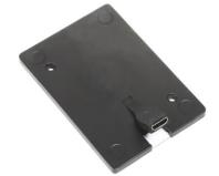
The new TWN4 Slim is ELATEC smallest compact and flat RFID reader – it's smaller than an ID-1 card. TWN4 Slim supports a huge range of LF and HF technologies (125 kHz and 13.56 MHz). With the support of NFC and Bluetooth Low Energy the reader supports mobile use cases for data communication and authentication. It can be operated as a standalone unit connected using a standard cable with a micro USB plug to PCs and other devices with USB interface.
