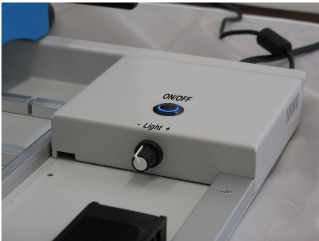
The power switch turns off the display, processor, and lighting. LED strip lighting is adjustable by potentiometer from 0 to 100%.
