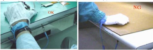
12.4 Please do not bend the film near the substrate glass.(this could cause film peeling and COF damage) and the peeling strength about 600g/cm, the bending <20times and the bending radius :R>0.8mm
