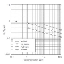
Fig3. Sensitivity characteristics
