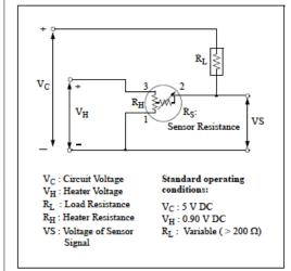
Fig 2. Standard circuit
