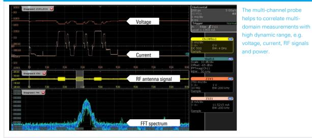
The extraordinarily high dynamic range allows the measurement of both active state currents and sleep currents, in this example 12 mA and 30 µA. Automated measurements make it possible to calculate the total energy consumption.
