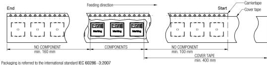
Projection 165° - 180° 2.5 SSt 2014-09-16 BD 2.4 2013-12-11 SSt SSt 2.3 SSt 2013-04-29 SSt Würth Elektronik eiSos GmbH & Co. KG EMC & Inductive Solutions 2.2 SSt SSt 2012-12-05 Max-Eyth-Str. 1 2.1 2012-10-25 SSt BD 74638 Waldenburg Germany Pull-of force 2.0 2012-09-03 SSt BD Tel. +49 (0) 79 42 945 - 0 Tape width | 16 mm | 0,1 N - 1,3 N www.we-online.com 1.0 ME 2009-08-07 Tape width | 24 mm | 0,1 N - 1,3 N eiSos@we-online.com DATE BY CHECKED
