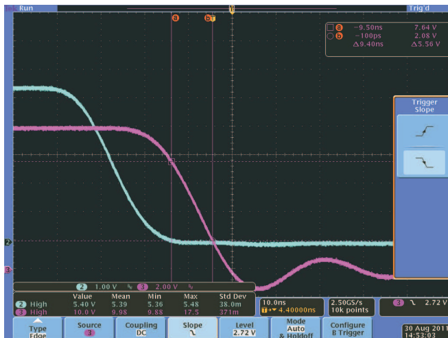
Figure 25. Typical Turn-On Waveform (VDD = 10 V, C L = 1 nF)
