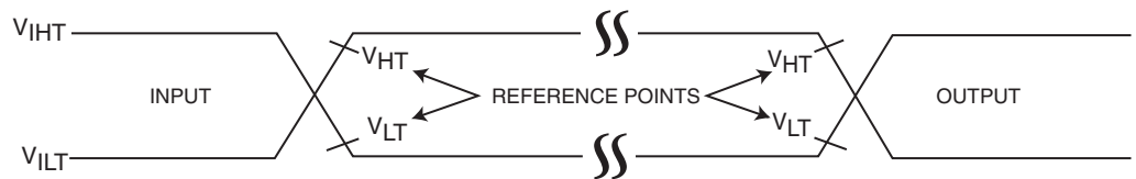
FIGURE 8-5: AC INPUT/OUTPUT REFERENCE WAVEFORMS
