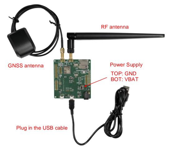
Figure 11: TE-B Wiring Diagram
