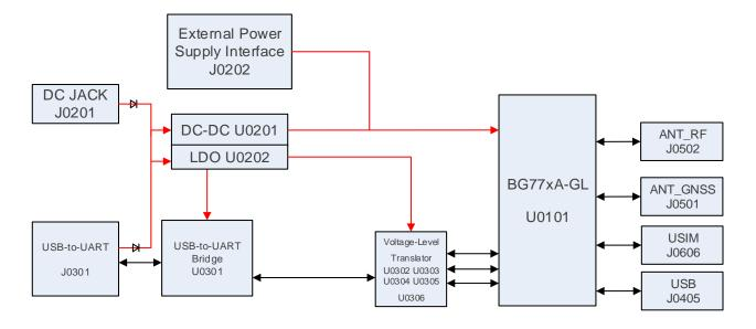
Figure 5: Functional Diagram of TE-B
