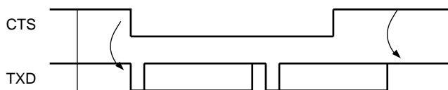
Figure 32-29. Transmitter Behavior when Operating with Hardware Handshaking
