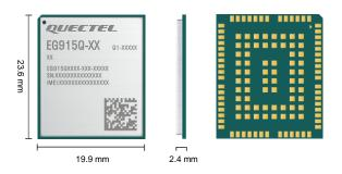
Quectel EG915Q-NA is an LTE Cat 1 bis module optimized specially for M2M and IoT applications. Adopting the 3GPP Rel-14 LTE technology, it delivers maximum data rates up to 10 Mbps downlink and 5 Mbps uplink. Designed in a compact and unified form factor, EG915Q-NA is compatible with Quectel LPWA BG95 series/BG96/BC95-G modules and LTE Standard EG91/EG95 series modules.
