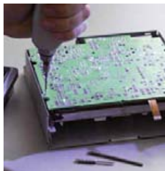
Halfmoon bits are always used for quick and precise work with miniature screws.
