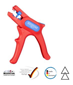
WEICON Wire No. 6 is an ergonomic automatic wire stripper. With the automatic scanning system, no adjustment to the cable cross-section is necessary. The fibreglass-reinforced wire stripper has an adjustable length stop from 5 - 12mm. This allows all solid and solid conductors from 0.2 - 6.0 mm<sup>2</sup> to be stripped efficiently and evenly. The fully insulated tool complies with the regulations on individual testing according to VDE IEC 60900 and withstands voltage up to 10 volts.
