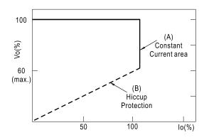
Typical LED power supply I-V curve
