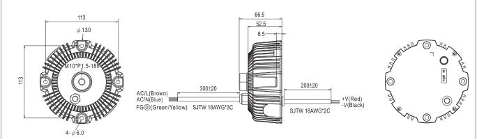
$\times$ IP65 rated. Output constant current level can be adjusted through internal potentiometer.
