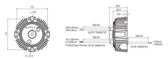
XIP67 rated, output constant current lever can be adjusted through output cable with 1-10V,PWM signal and Resistance
