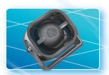
The SAS-325A-6 is a universal electromagnetic siren with very high sound output. At 30cm the sound pressure level is about 123 dB(A). Six different alarm tones can be programmed by jumpers selection, which enables the user to choose and pre-select an alarm function for different application fields.
