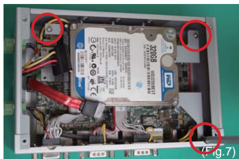
7. Screw the HDD Kit to the system with 3 x flat-headed (M3*4) screws. (Fig.7)
