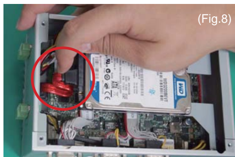
8. Connect the SATA DATA Cable to HDD. (Fig.8)
