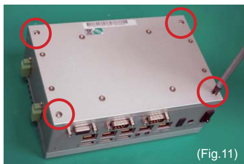
11. Screw the top cover to the system with 4 round-headed M3*5 screws. (Fig.11)
