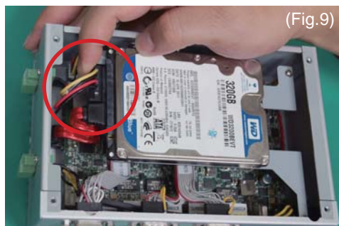
9. Connect the SATA Power Cable to HDD. (Fig.9)
