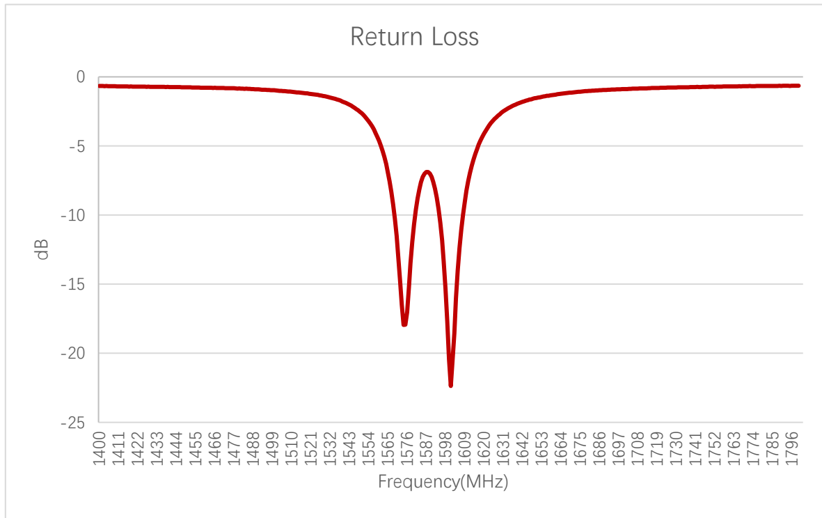
Return Loss (dB) – GNSS
