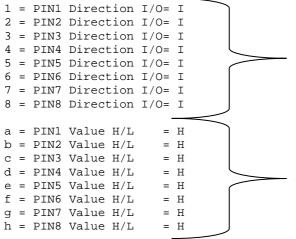
Using these settings, it is possible to determine if the single PINs shall act as input or output when starting the interface. It is also possible to set this function via the protocol during operation. Please find an explanation on the following pages.
