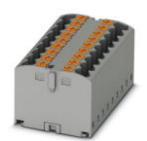
Distribution block, Basic terminal block, connection method: Push-in connection, number of connections: 12, cross section:0.14 mm² - 4 mm², AWG: 26 - 12, width: 31.2 mm, height: 21.2 mm, color: blue, mounting type: adhesive
