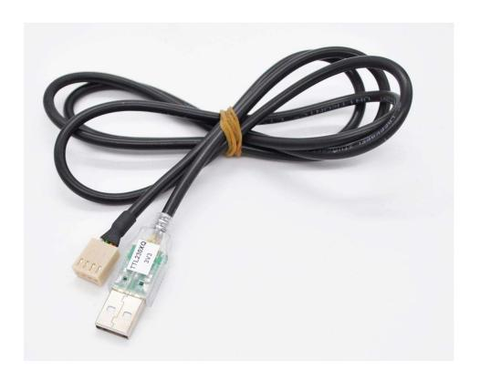
Figure 1 - The TTL-230XQ-3V3(5V) USB to TTL Serial Converter Cable
