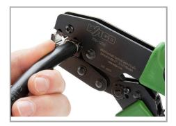
Squeeze handles until ratchet mechanism is released.
